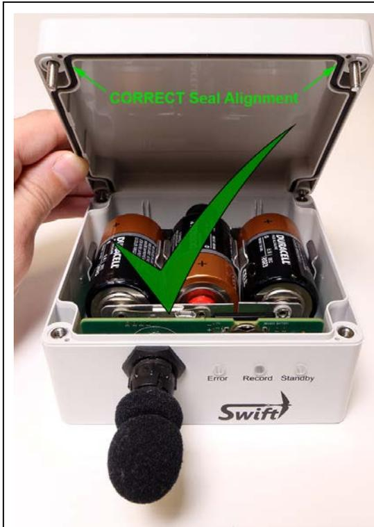
When the lid is oriented correctly, the rubber seal aligns with the ridge on the lower half of the enclosure
