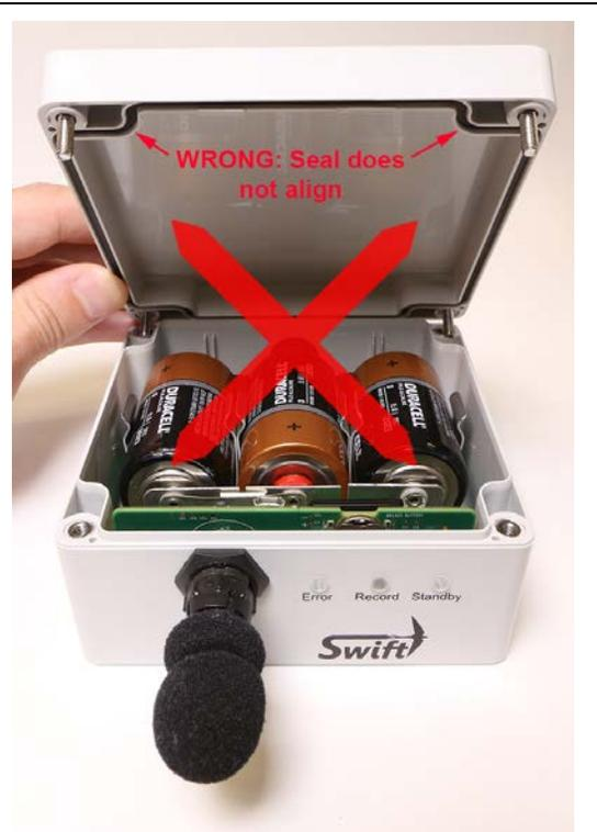
This image shows an improperly aligned lid. The rubber seal does not match up with the lower half of the enclosure. Rotate the lid 90 degrees in either direction for proper alignment
