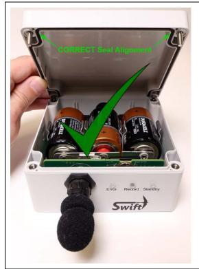
When the lid is oriented correctly, the rubber seal aligns with the ridge on the lower half of the enclosure
