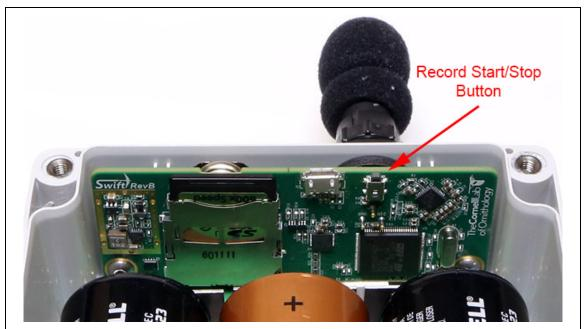
Push and hold the Record Start/Stop button for approximately two seconds to switch between Record and Standby Modes.
