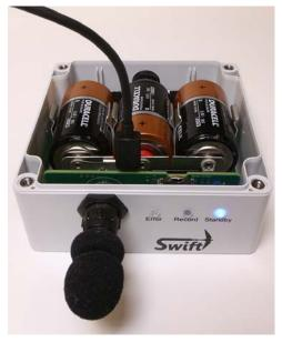
To configure Swift, plug a micro USB cable into the usb connector as shown
