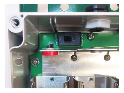
When the switch is turned to the "Power On" position, the LED's on the front of the enclosure will flash to indicate it's current operating state.
