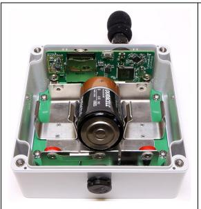
Insert center battery first with positive battery terminal against red ringed contact on battery holder
