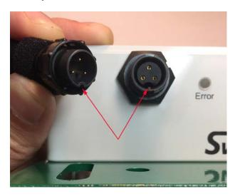
Once the microphone is aligned, push the two halves firmly together. Then rotate the threaded sleeve in the clockwise direction until it locks into place.
