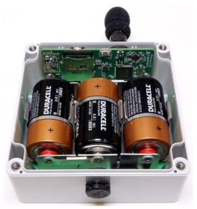
Install two side batteries in the same way
