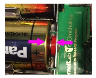
The battery holder slats may be bent back into position by using your fingers to put pressure on them as shown below. This process must be done with the batteries removed.
