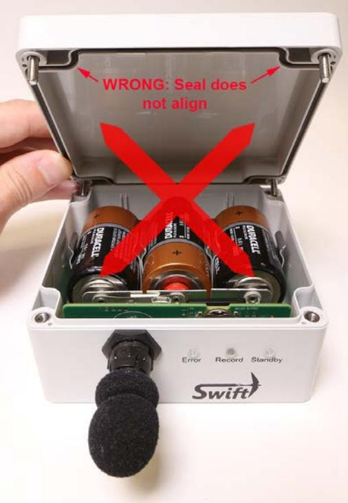
A photograph of the same Swift device with its lid open. Inside, four Duracell batteries are visible. A large red "X" is overlaid on the image, pointing to the top edge of the lid where it fails to meet the enclosure. The text "WRONG: Seal does not align" is written in red at the top center of the lid area. |
