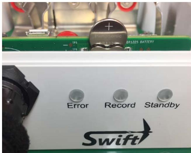
Push the battery down until it's fully seated in the holder as shown here:
