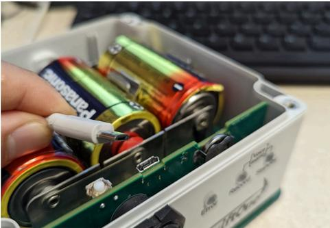
3. The SwiftOne recorder should light up the blue LED when connected to the computer. The program should automatically detect that a SwiftOne Device is connected. It should also show what version of the firmware the unit has. If the SwiftOne recorder is not detected, check the USB Cable that it's a data + power type. Try a different cable known to work with the SwiftOne Configuration Utility.
