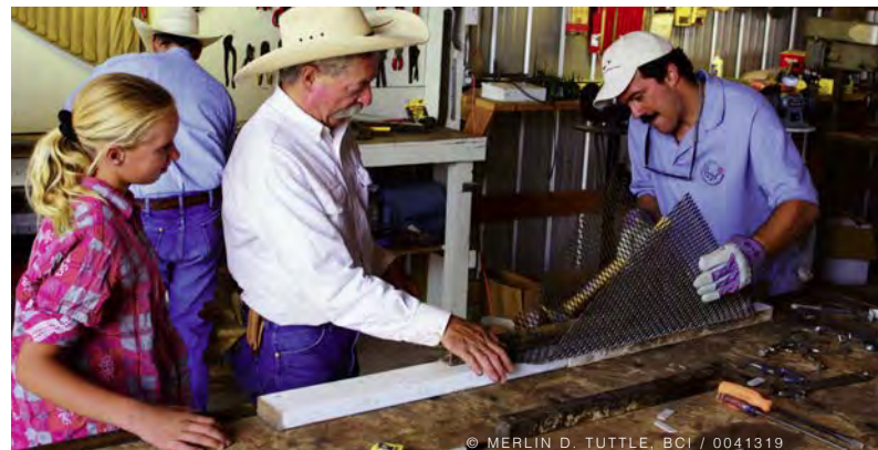
Dan Taylor (right) helps Dennis Moroney and his daughter, Ally, of the Cross-U Ranch in McNeal, Arizona, complete an expanded-metal escape structure by bending the sides to a 90-degree angle.
